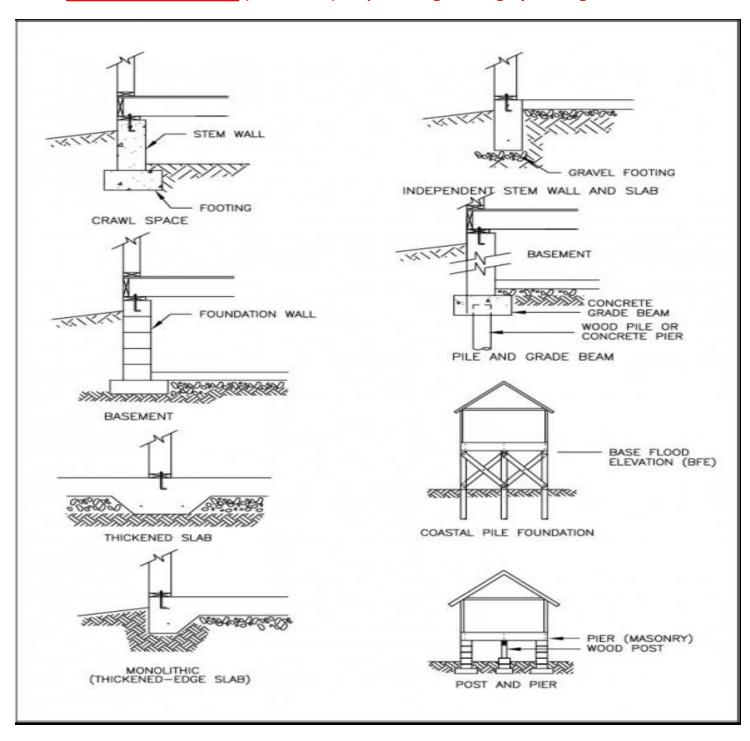
Provide Foundation Details in accordance with IRC or prescriptive method:
